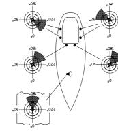
different positions after having installed the winch. other models, the selftailing arm can be placed in several location of the holes prior to drilling these in the deck. On all arm is fixed, making it very important to establish the proper shaded area. On 12ST and 28ST the position of the selftailing recommend to have the selftailing arm positioned within the Be also aware that selftailing arm is positioned correctly. We
