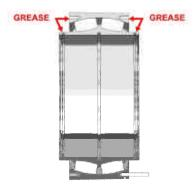
Fit each V-seal and seal carrier.
