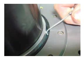
With the tool supplied, hook the inner edge of the seal to provide access to the rollers.
