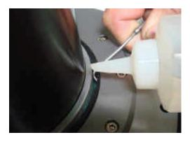
Add a few drops of the silicone oil supplied through the gap in the seal. Rotate the rudder back and forth to help distribute the oil through the bearing. The oil
