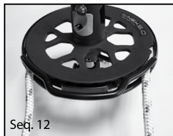
Drosse installée / Installed furling line
